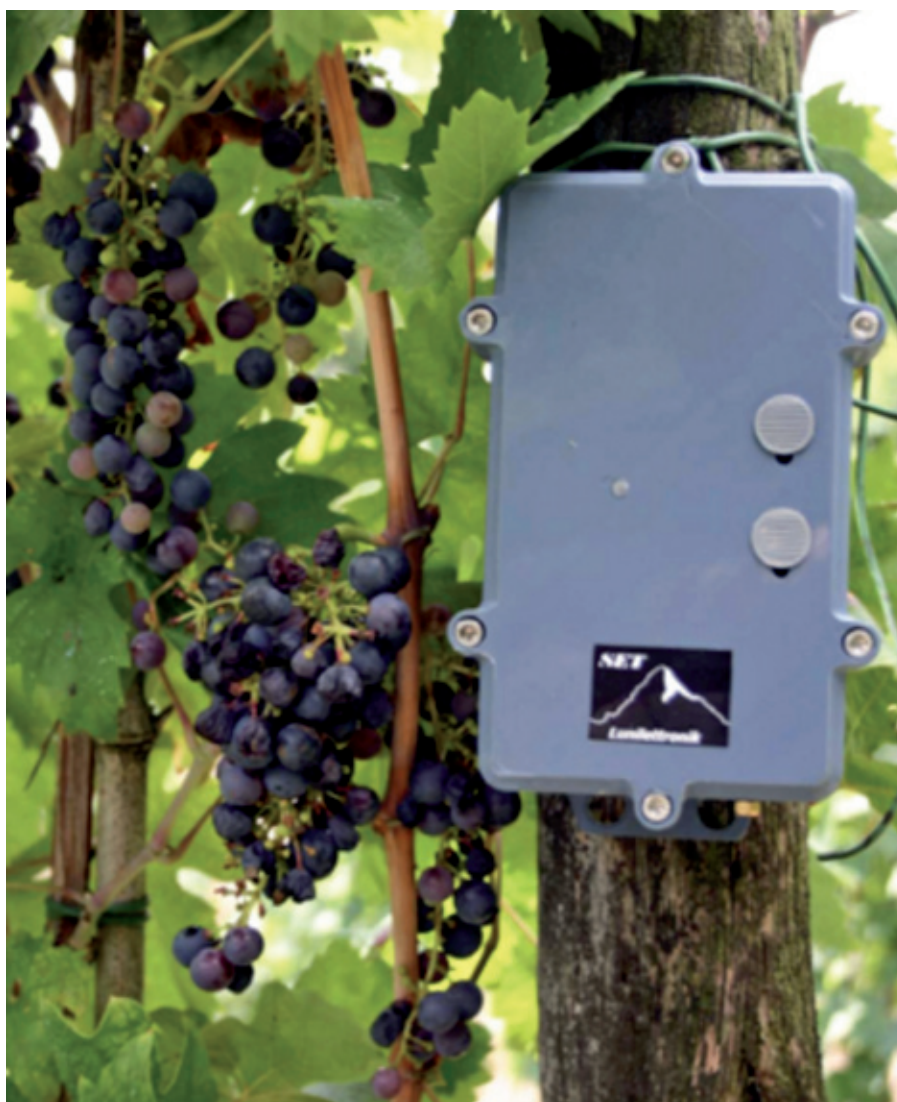
Fig. 1 – A Soundscape Explorer [Terrestrial] SET tied to a pole for vineyards. The small size (12x20x6 cm) allows to easily place this device in the wild (credit: Almo Farina, IInstEco).
