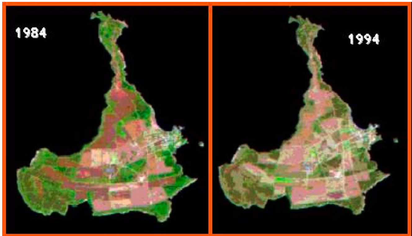
Figure 5 – Normalized Difference Vegetation Index (NDVI) of Pianosa in 1984 and 1994, showing a decrease in overall vegetation index associated to human activities. The dark and pale green areas represented the Mediterranean ecosystems, while the red and brown areas represented tilled and pasture areas. White areas are buildings and roads.
